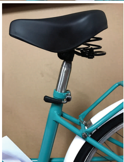
No 6: Adjusting the saddle height
