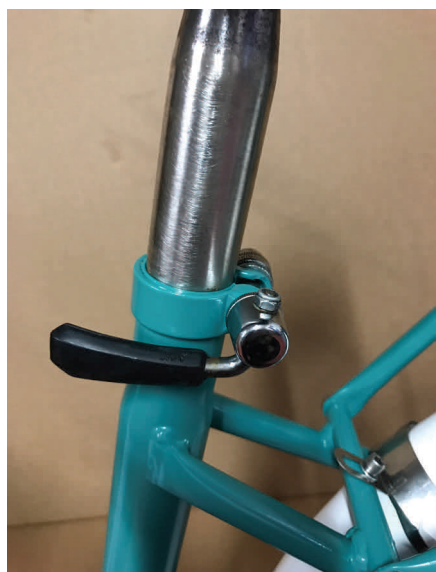
No 5: Quick Release Adjustor
